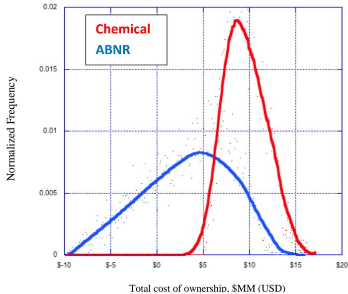
FIGURE 3: MONTE CARLO SIMULATION OF ABNR VS. CHEMICAL SOLUTION
