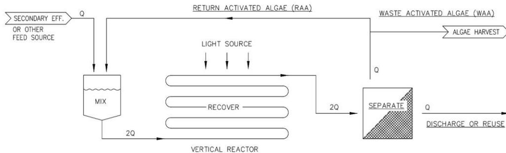
FIGURE 1: HIGH-LEVEL ABNR PROCESS FLOW
